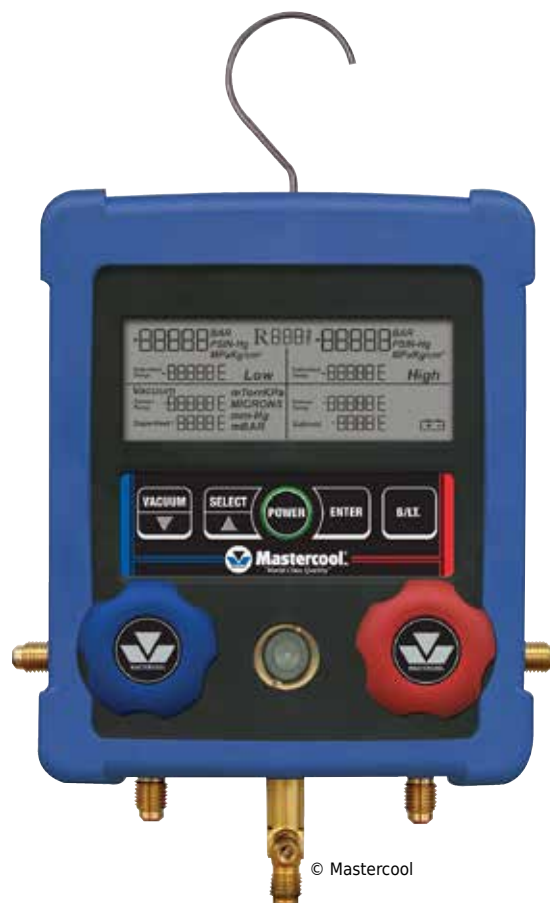
Electronic manifold gauge set that can be used with flammable refrigerants
