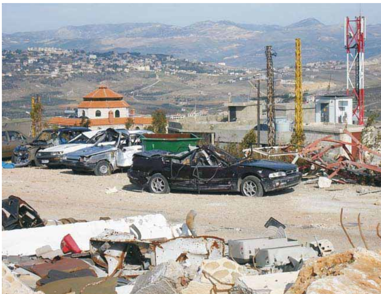
Burnt car batteries are likely to be the source of elevated lead concentrations at the site of the former Khiam prison
