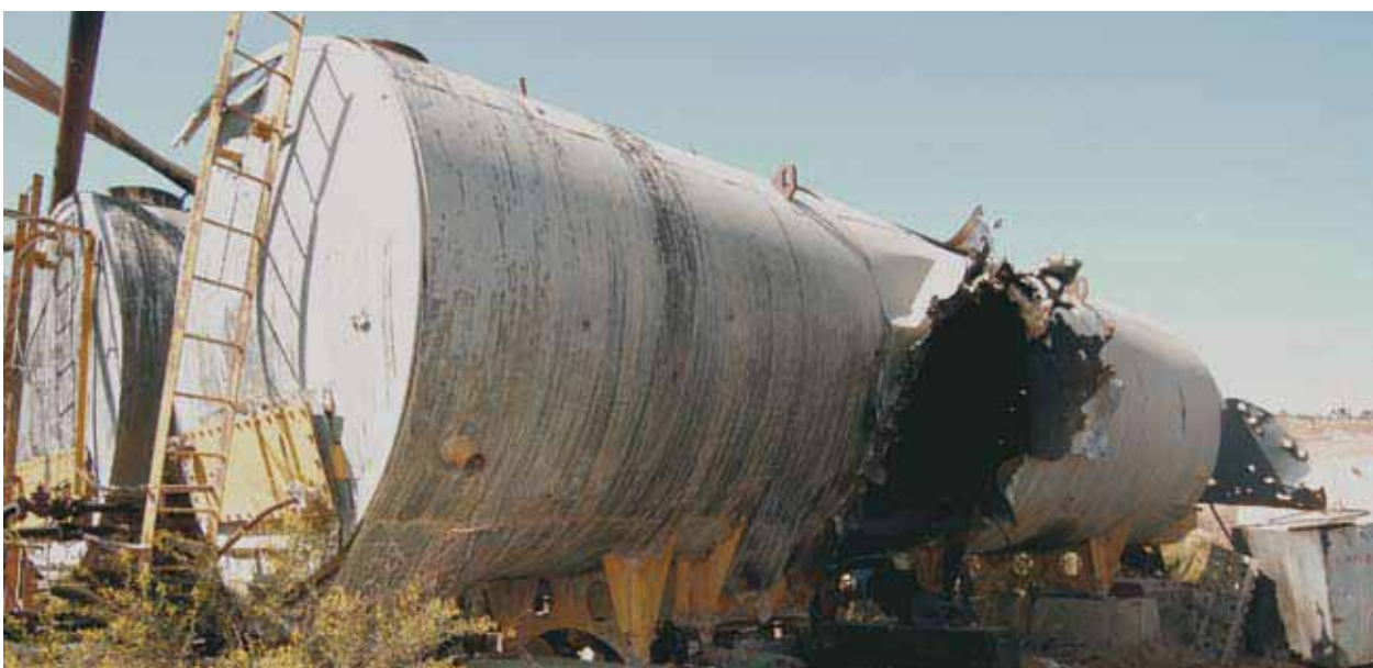
A damaged diesel tank in the Ebl Saqi asphalt plant
