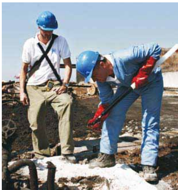
UNEP expert extracting groundwater sample at Jiyeh power plant using a portable bailer
