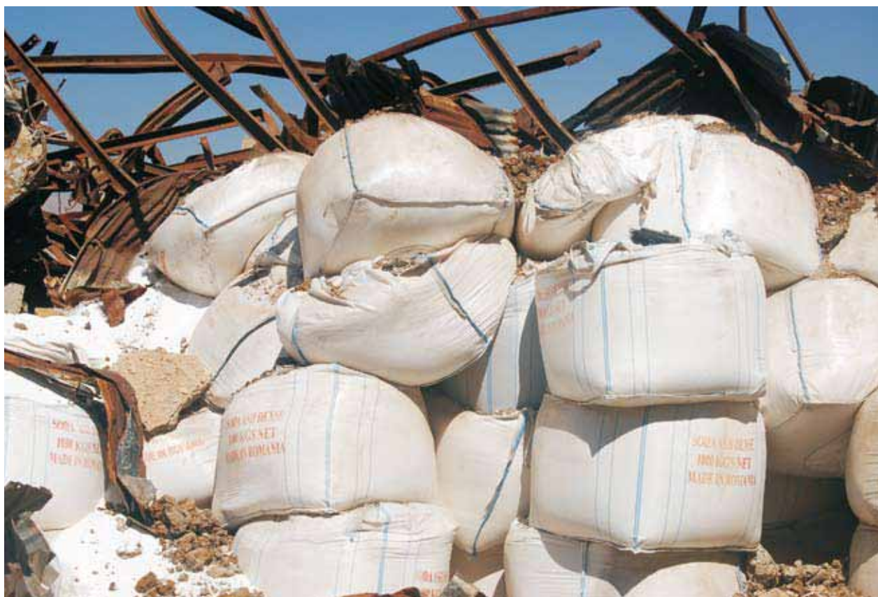
Chemicals used in glass production will leach into the groundwater unless relocated under cover
