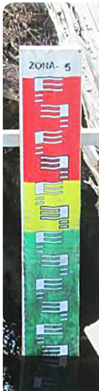
Figure 15. Measuring Water Level
