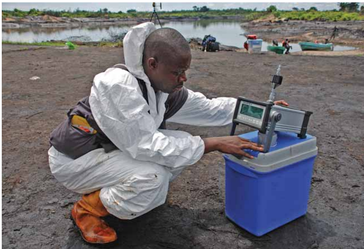
A Thermo Scientific Particulate Monitor DataRAM 4 is used to measure air quality, Bodo West
