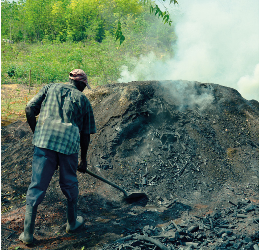
Photo 1. The process of making charcoal typically takes around 4-5 days, whereby all water and volatile elements of freshly cut wood becomes converted to carbon through a slow pyrolysis method. The traditional charcoal production method includes a pile of wood covered with dirt and leaves that will be lit from below and left to burn. This method of charcoal production is highly inefficient from an energetic perspective, as only around 25% of the energy in the wood remains in the finished charcoal.
