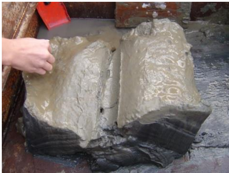
Figure1: Muddy sediment sample taken with a large grab sampler. The top 1 cm layer is collected for chemical pollution analyses. The oxic and anoxic layers can be clearly observed,
