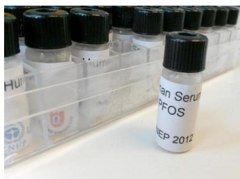
Figure 5: Test samples were ampouled and shipped to laboratories; here: PFAS standard solution and human serum for PFOS analysis Photo courtesy of Dr. Bert van Bavel, MTM Research Centre, Örebro University, Sweden
