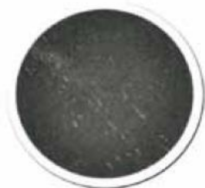
Retrofitted with Diesel Oxidation Catalyst (DOC) (Level 1)
