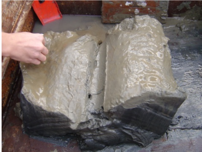
Figure 1: Muddy sediment sample taken with a large grab sampler. The top 1 cm layer is collected for chemical pollution analyses. The oxic and anoxic layers can be clearly observed, Image provided: Mudsedimentsample_CGuitart.jpg
