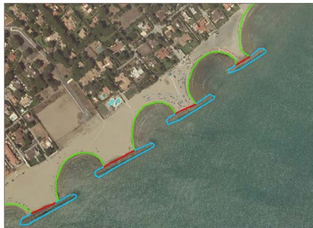
Figure 2. Image showing coastal defence structure (blue), artificial coastline (red) and natural coastline (green) (image developed by G.Giorgi)
