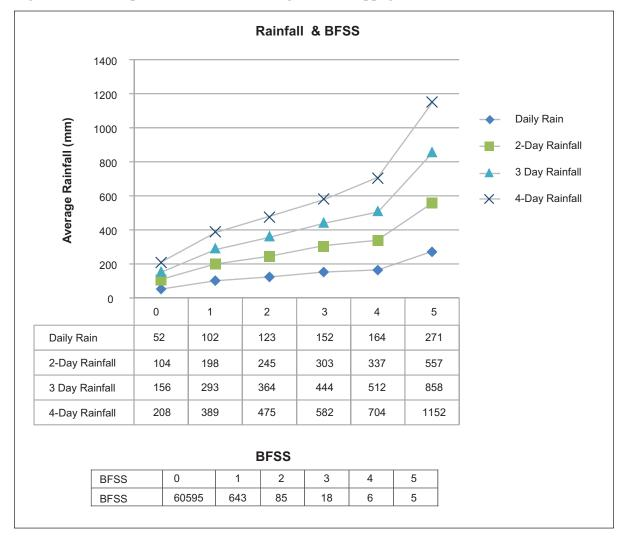
Figure 8: Rainfall pattern on boulder falling and soil slippage
