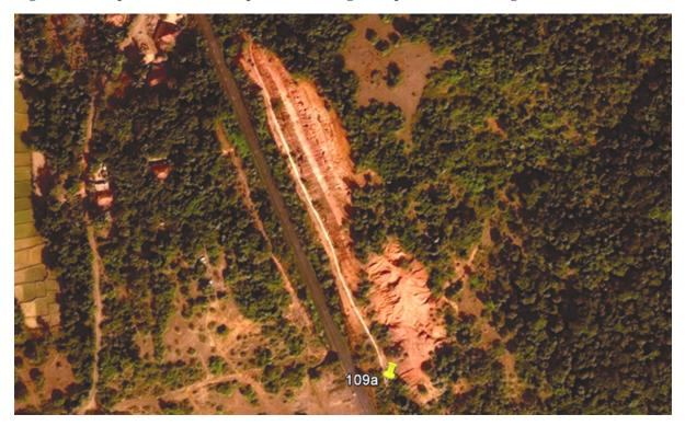
Figure 10: Adaptation work example – Flattening of slope is visible on right side of track
