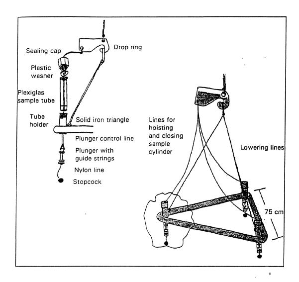
Figure 1. Three-core Albrechtsen bottom sampler.
