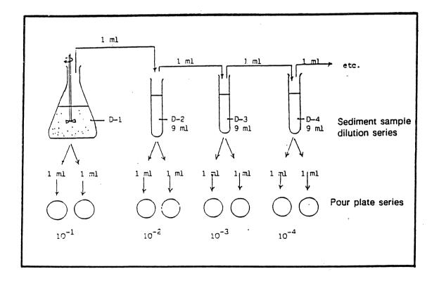
Figure 3. Working diagram for the determination of faecal coliforms in sediments by the Pour Plate method.
