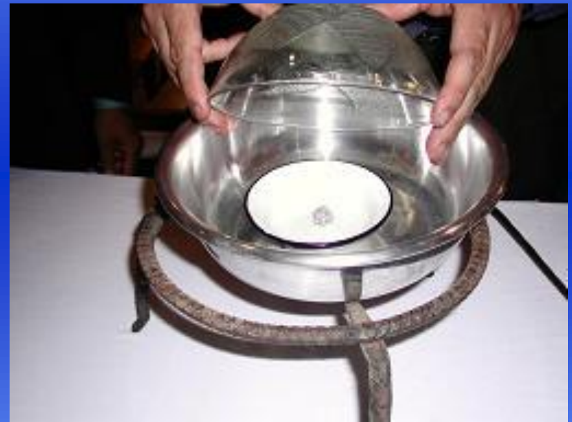
Simple and cheap retort easy to procure locally UNIDO-GMP, Laos, 2003
