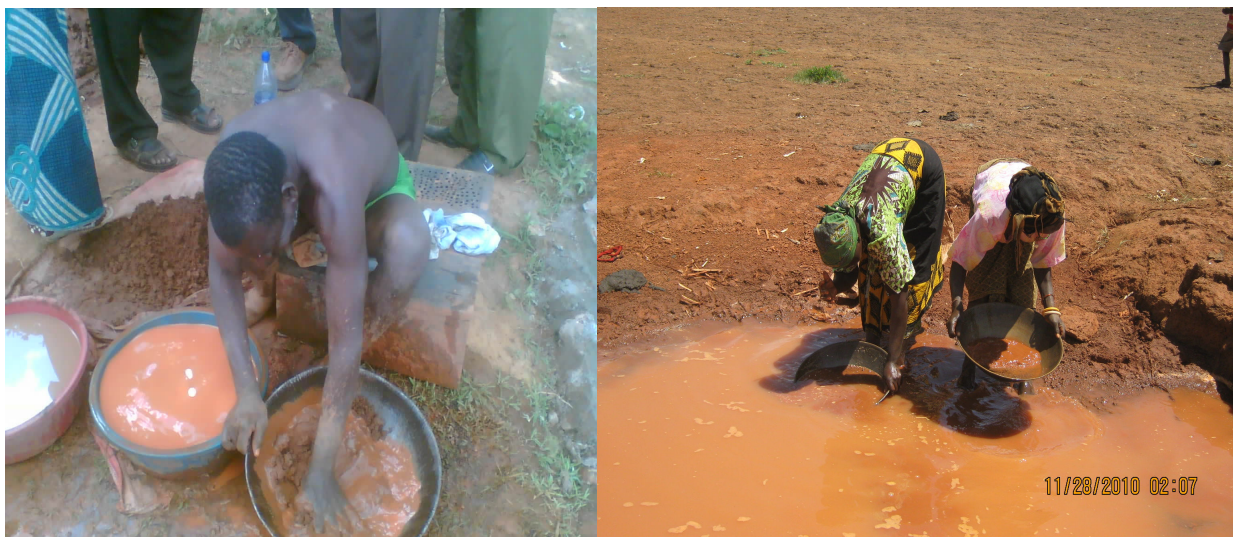
Figure 4: Illustrate ore amalgamation with mercury
