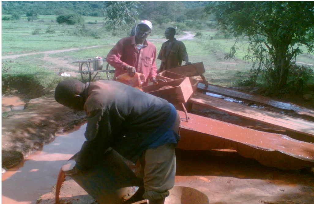
Figure 3: Gold extracted using local table
