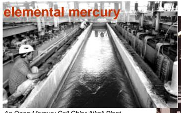
An Open Mercury Cell Chlor Alkali Plant Source: Centre for Science and the Environment, New Delhi, "Down to Earth"
