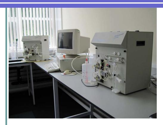
Cold Vapour Atomic Fluorescence Spectrometry (CV-AFS)
