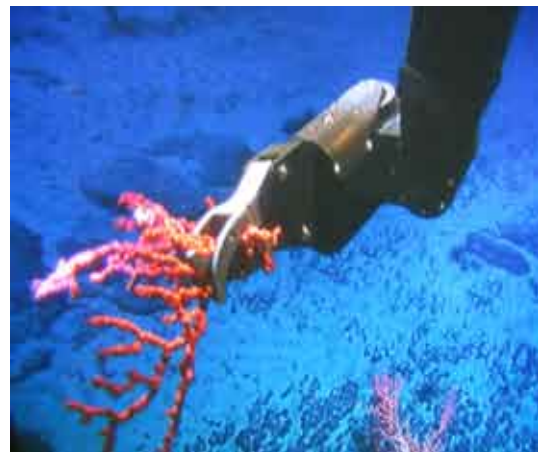
Sampling a small coral colony with ROV Hercules manipulator arm. Photo courtesy of M. Grady NOAA Ocean Explorer
