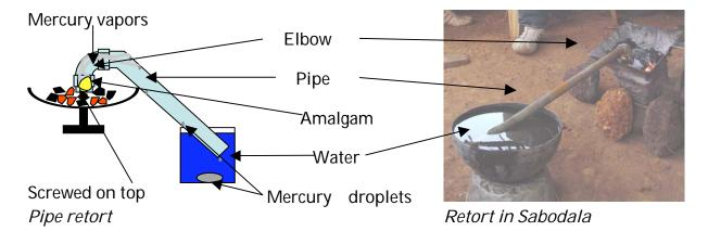
This retort is the easiest easy to make, efficient and inexpensive. It had the most success with the miners during the field training sessions. The small contact surface area that touches the fire, leads to a high exchange of heat and the sublimation of mercury is accelerated. Because each item used is a plumbing item, they can be screwed together creating a very tight seal. This captures the mercury vapors really well.
