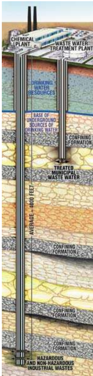
Figure 28 Outline of deep well injection (source: US EPA)
