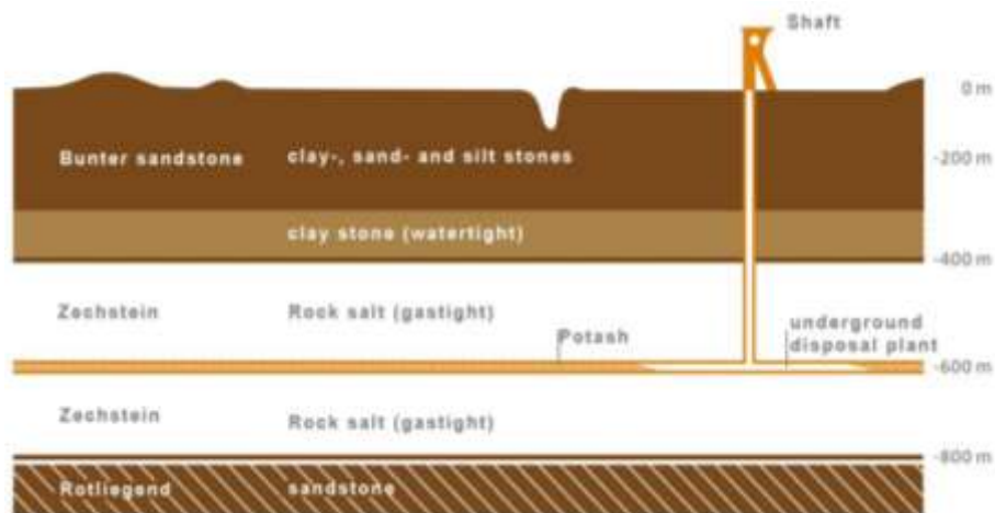
Figure 45 UTD 15 Herfa-Neurode, geological cross section of the site (source: K+S Entsorgung [4])
