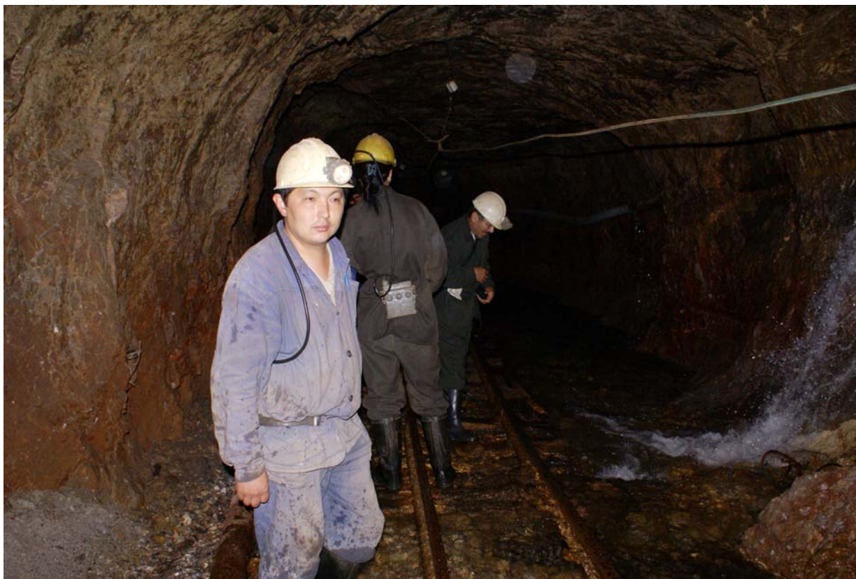
Figure 13 Khaidarkan mine: Vspomogatelnaya shaft (400 m). Carstic water intrusion
