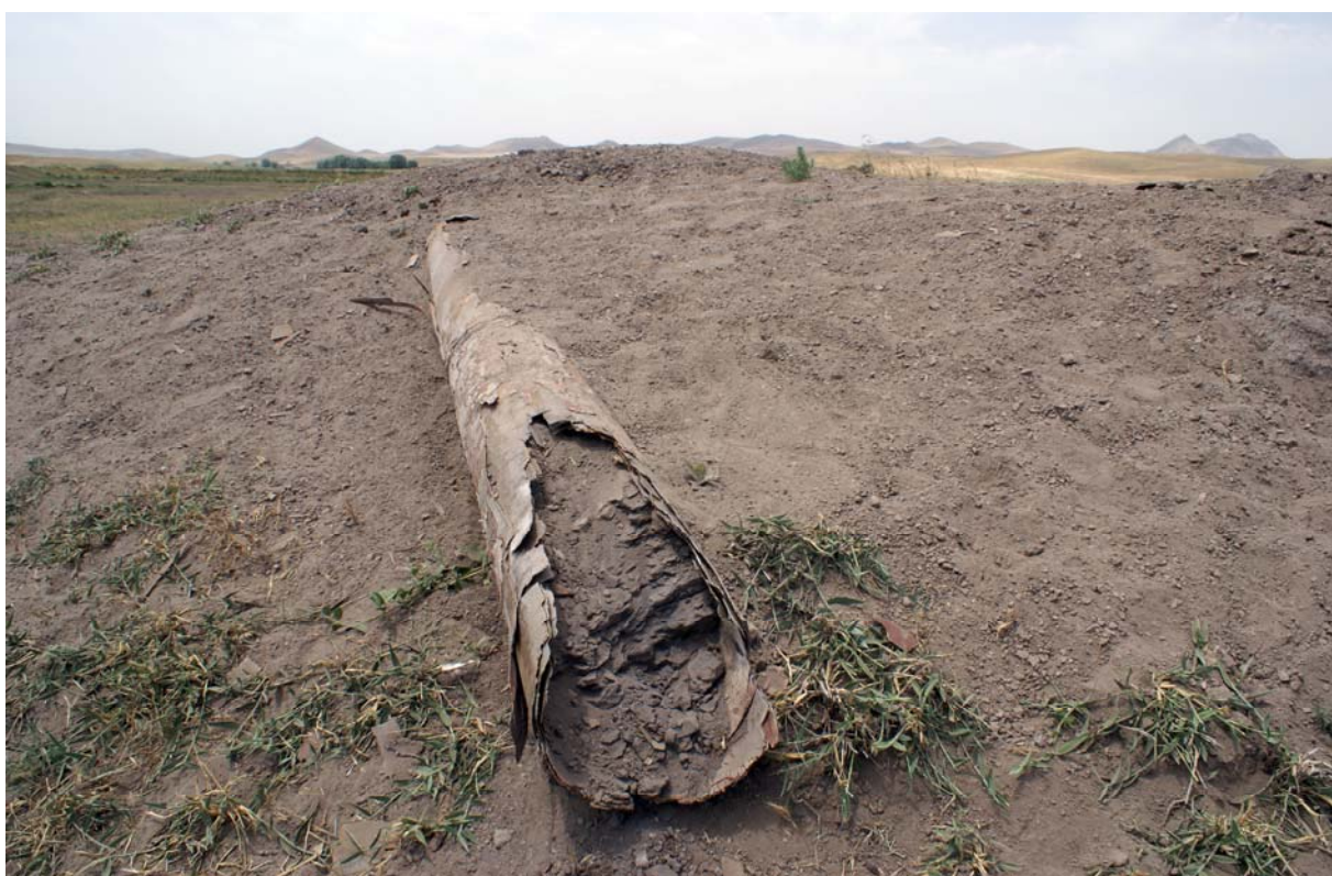
Figure 28 Chonkoy-Ulug-Too mine: dry tailings and wastepipe
