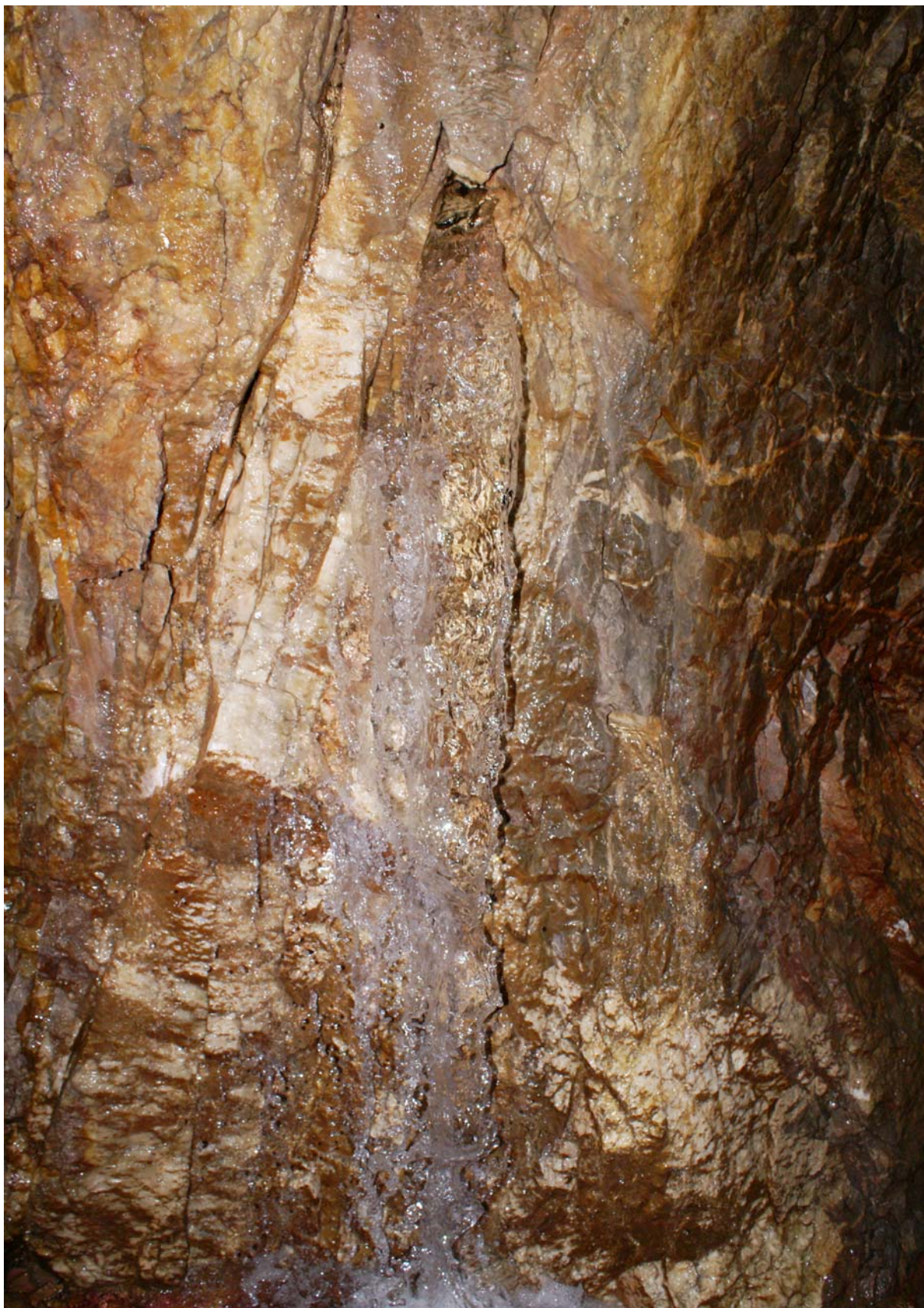
Figure 15 Khaidarkan mine: Carstic water intrusion. July 2008
